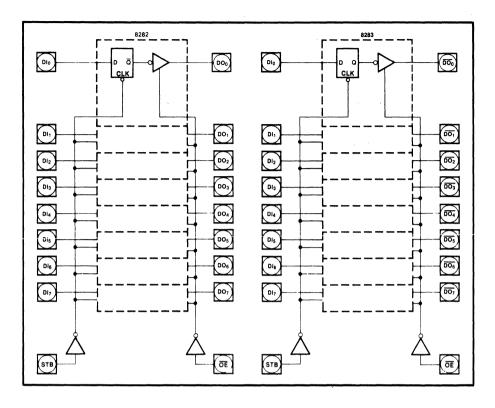
Figure 3. Logic Diagrams
